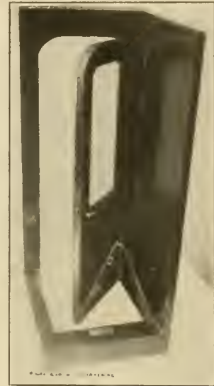
VESTIBULE DOOR WITH SELF OPENING TRAP DOOR.
